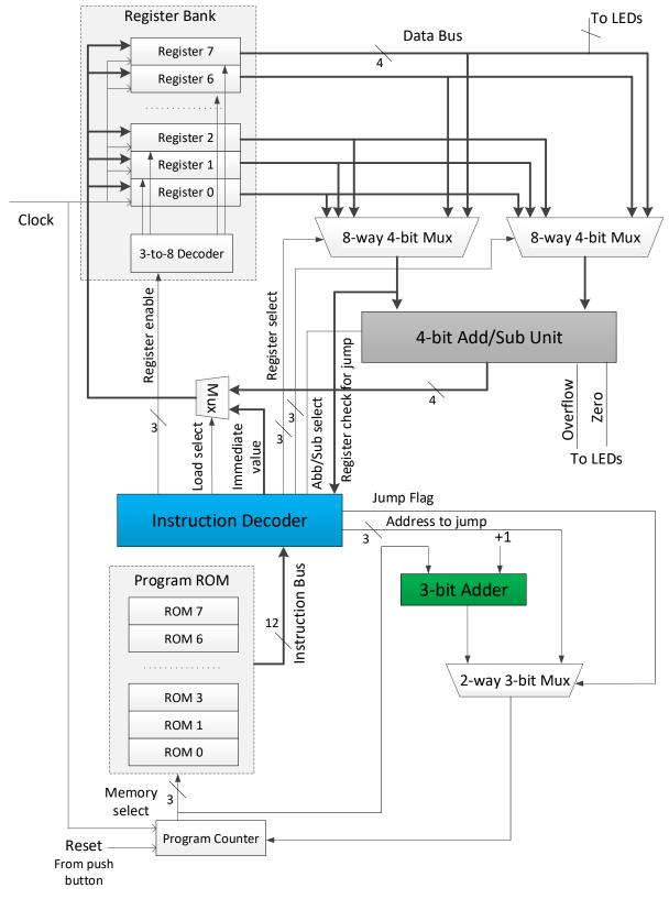
Figure 1 – High-level diagram of the nanoprocessor.
