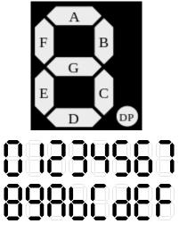
Depending on the number we want to display, we can switch on or off the desired segment(s). Which segment you may want to switch on or off also depends on the specific 7-segment implementation, where it may light up depending on an active high (common cathode circuit) or active low input (common anode circuit).
