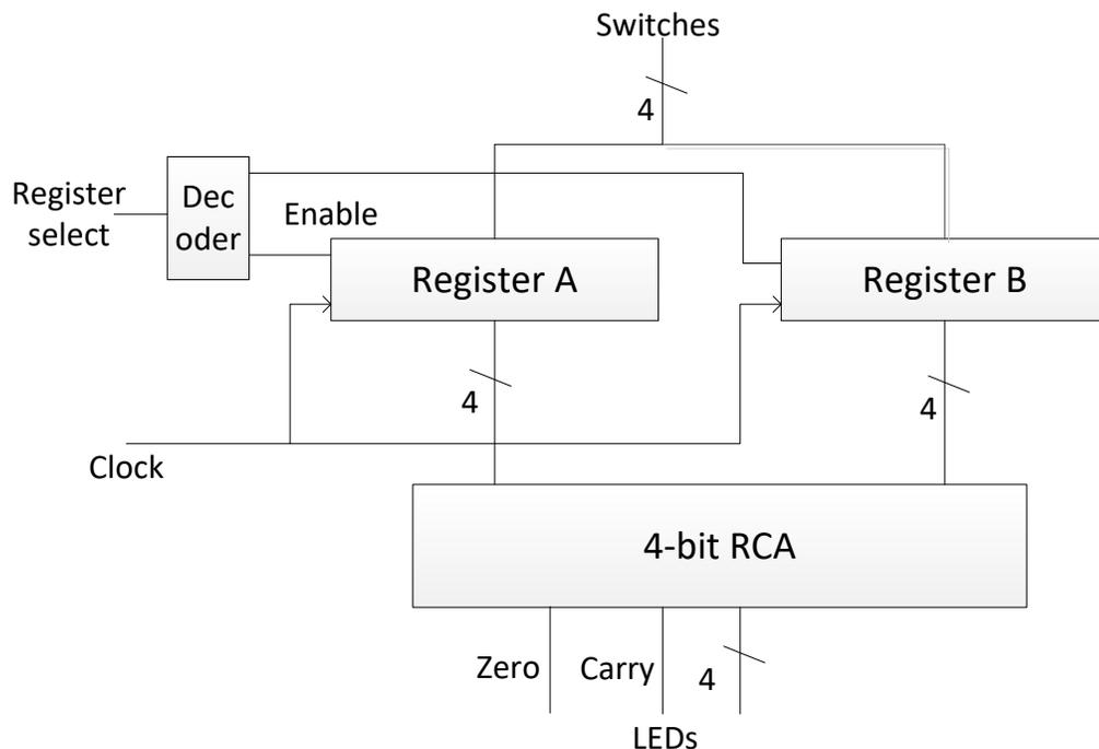
We will build a 4-bit register using D Flip Flops. Register also has an Enable input and a Clock input. 2 registers are then connected to our 4-bit Ripple Carry Adder (RCA) developed in Lab 3. This forms a simple AU.
