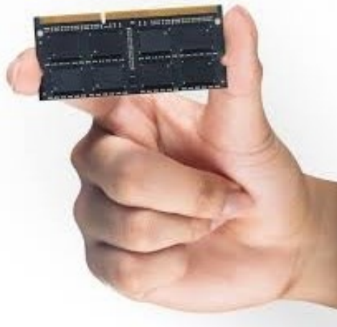
Figure 18 – How to hold a circuit board.
