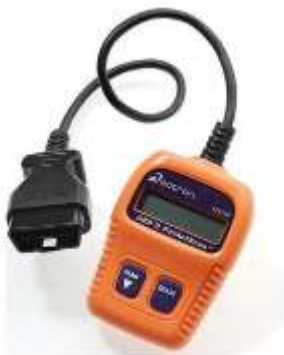
Figure 2.1. A handheld OBD2 scanner (Actron PocketScan) [14].
