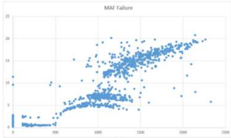
Fig. 3.4 The Engine RPM vs the MAF value of the collected dataset
