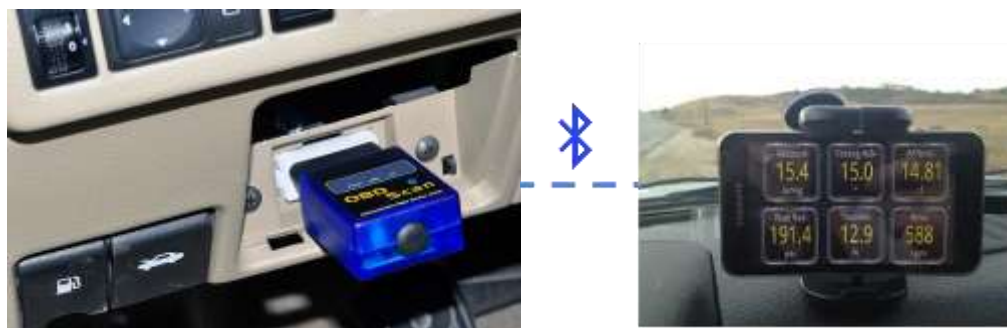
Figure 2.3. Reading data using an OBD2 Bluetooth adaptor and a mobile phone [16].
