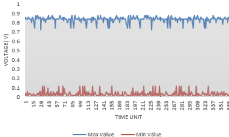
Fig. 3.1. Min max variation of a healthy O2 Sensor.
