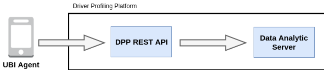
Figure 3.7: Vehicular data publisher service flow diagram.
