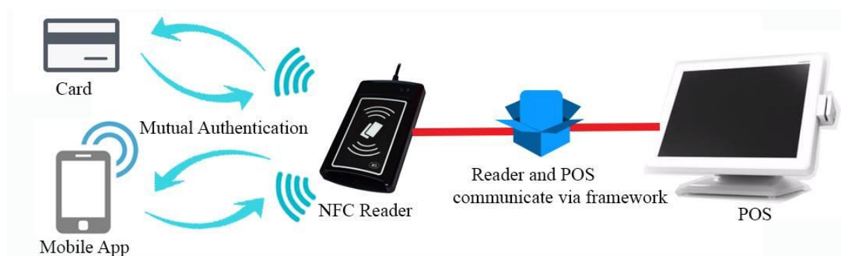
Figure 1.1 Targeted project deliverables, which include four main modules; NFC card, reader, mobile application and libraries for the framework
